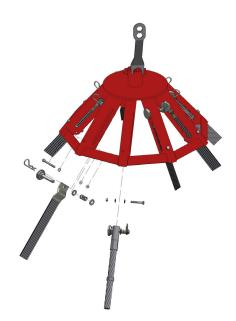
The weed brush can operate with two different brush types: The standard flat steel brush and a wire brush. If you want to switch from the flat brush to the wire brush, unscrew the M6x60 machine bolt located at the base of the brush profile and tighten a new M6x40 machine bolt through the other  $\emptyset$ 7 hole in the brush profile before inserting the brush.
