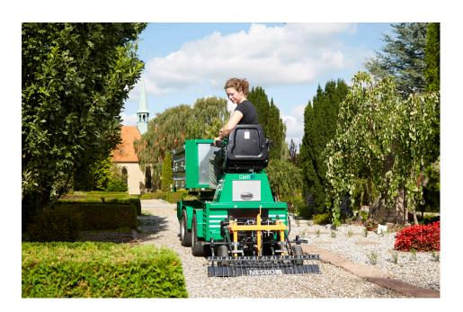
At the end of the season, clean the Weed grater and remove weeds, soil and the like. To prevent rusting, wipe the moving parts (but not the motor) with oil.
