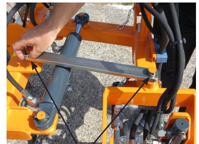
Remove the 2 ring pins on the steering rod. Remove the steering rod.
