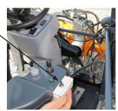
Tractor equipped with 1 dual hydraulic connection.
