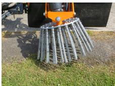
There are several different brush head settings, which determine different directions of spread.
