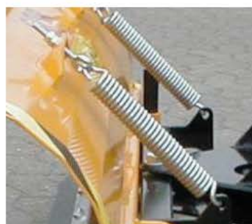
Spring arrangement for securing the blade at collision
