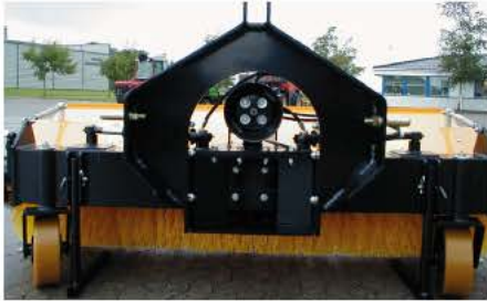
Swingspeed gearbox for tractors with high PTO speed
